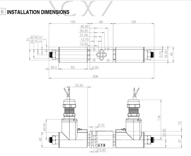
All valves HD3-\* conform with ISO and CETOP specifications for mounting surface dimensions (see also front page) and for valves height. When assembled to its mounting plate valve HD3-\* must be fastened with 4 bolts M5 X 45 mm (or M5 x \*\* according to the number of modules) tightened at 8 Nm torque. Leakage between valve and mounting surface is prevented by the positive compression on their seats of 4 seals of QUAD/O Ring type 9,25x1,68x1,68.
