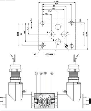
The spool 12 shifts into the valve body 11 subject to the action of springs 13 and solenoids 2. Spool 12, depending from its shape and its position in the valve body, opens and/ or closes passages between P, A, B and T ports, thus controlling the direction of the hydraulic flow.
